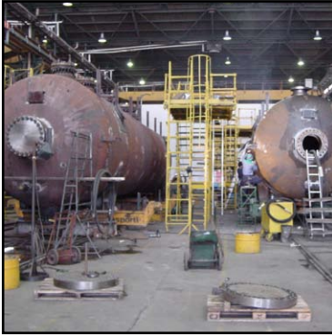
Two of the slug catchers ready for internal coating.
