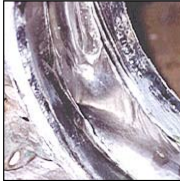
Abraded end suction casing
