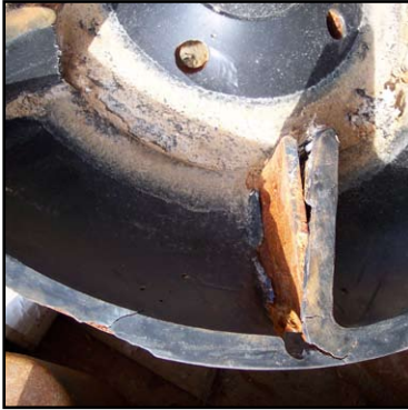
Typical wear from oil well service caused by sand/water at high pressure
